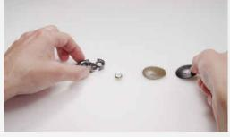
2. Remove the cover completely from the audio processor. Place the new cover on the Samba by positioning the rear side of the cover on the audio processor first. Press the cover down: firstly on the rear side, then on the front side. Make sure that it snaps into place.
