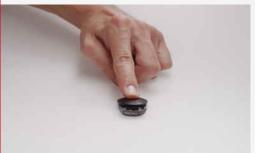
1. First, remove the battery (see above). Then place the Samba on an even surface such as a table and put one finger on top. First, lift one side of the cover then lift the other side.
