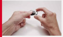
1. To change the battery, hold the device between two fingers. First open one side of the battery case, then open the other side.
