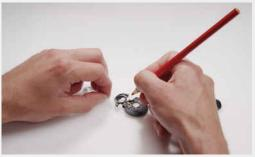
2. Feed the attachment thread through the small notch under the battery case. Press the attachment thread down to fixate it in the audio processor. Use a small pointed object such as a pencil for doing this.
