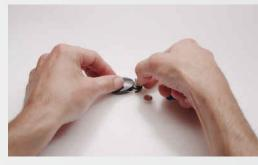
3. Take a new battery and remove the sticky tab from the top. Place the battery in the audio processor's battery case. To activate the Samba, slide the battery case into the audio processor with two fingers.
